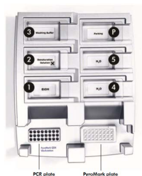
Figure 5. Placement of PCR plate (or strips) and PyroMark Q24 Plate on the PyroMark Q24 Vacuum Workstation. The marked positions contain 70% ethanol (1), PyroMark Denaturation Solution (2), PyroMark Wash Buffer (3), and high-purity water (4, 5). P: Parking position.
