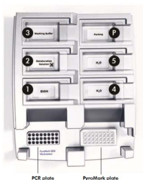
Figure 23. Positions on the PyroMark Q24 Vacuum Workstation.
