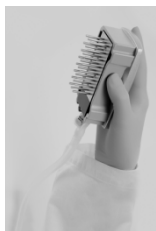
Figure 10. Illustration of the vacuum tool raised to beyond 90° vertical.
