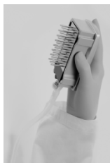
Figure 6. Illustration of the vacuum tool raised to beyond 90° vertical.
