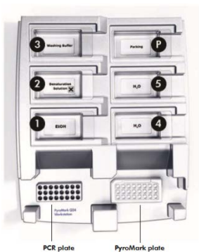
Figure 9. Placement of PCR plate (or strips) and PyroMark Q24 Plate on the PyroMark Q24 Vacuum Workstation. The marked positions contain 70% ethanol (1), PyroMark Denaturation Solution (2), PyroMark Wash Buffer (3), and high-purity water (4, 5). P: Parking position.
