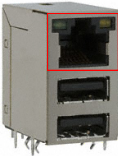
Figure 2a. Ethernet Port
