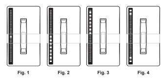
The transition status display at the left side of the fader lever indicates not the lever position but the amount of transition, and also works during auto transition
