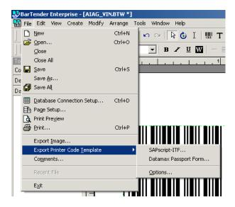
You can export a printer code template as one file or you can break it up into format and data printer code. Typically printers can accept printer code of two different types:
