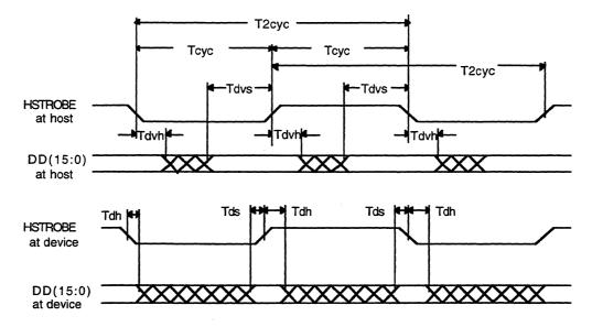
Figure 6-9 Sustained Data Out Burst
