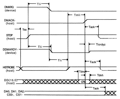
Figure 6-11 Host Terminating a Data Out Burst
