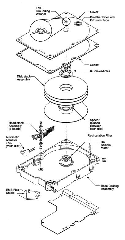
Figure 5-1 Quantum Fireball CR 4.3/6.4/8.4/12.7AT Hard Disk Drive Exploded View
