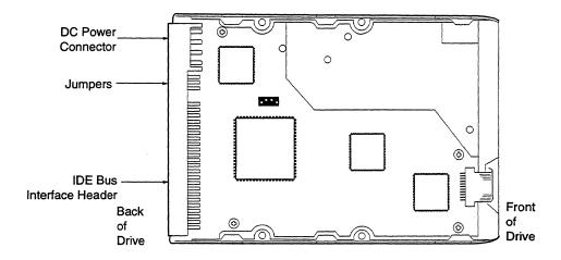
Figure 3-4 Jumper Locations for the Quantum Fireball CR Hard Disk Drive
