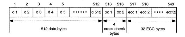
Figure 5-5 Sector Data Field with ECC Check Bytes
