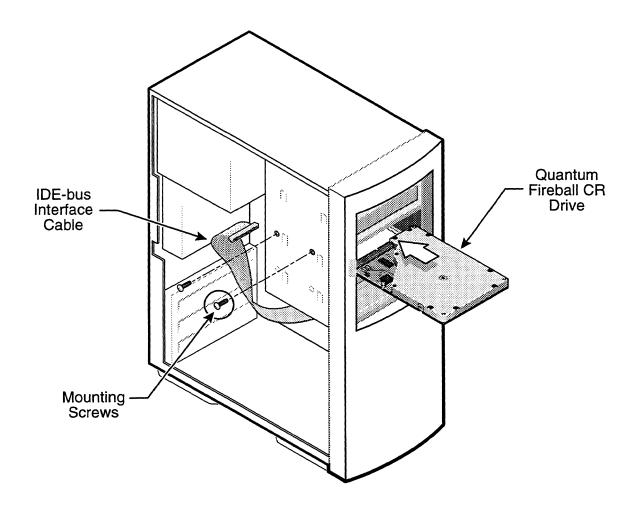
Figure 3-12 Completing the Drive Installation
