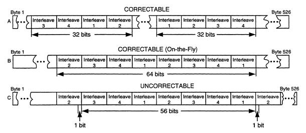
Figure 5-7 Correctable and Uncorrectable Double-Burst Errors
