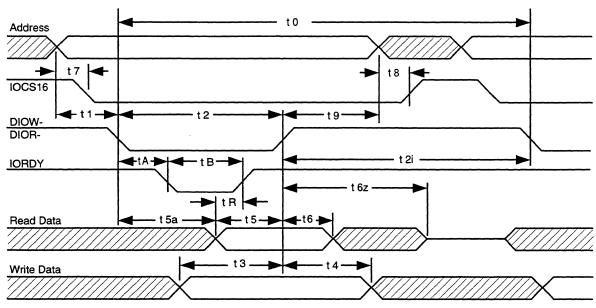
Figure 6-1 PIO Interface Timing
