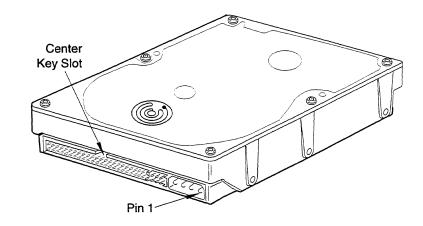
J1 IDE (40-Pin)/DC (4-Pin) Combination Connector
