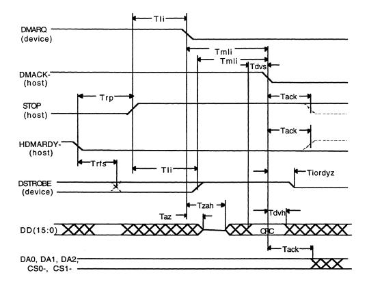
Figure 6-7 Host Terminating a Data In Burst
