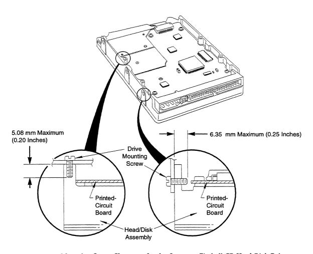
Figure 3-8 Mounting Screw Clearance for the Quantum Fireball CR Hard Disk Drives
