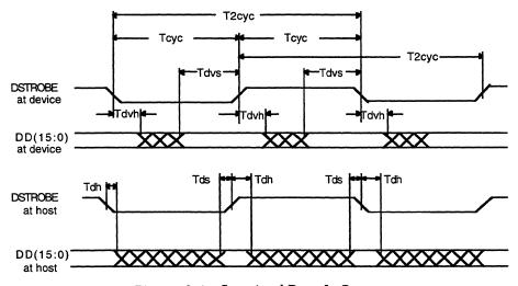
Figure 6-4 Sustained Data In Burst
