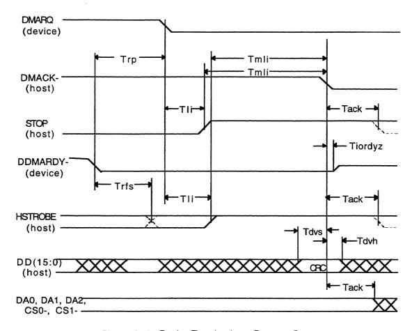
Figure 6-12 Device Terminating a Data out Burst
