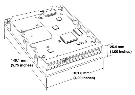
Figure 3-1 Mechanical Dimensions of Quantum Fireball CR Hard Disk Drive
