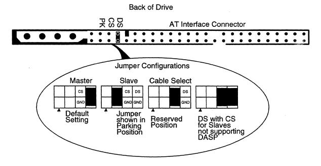
Figure 3-5 Jumper Locations on the Interface Connector
