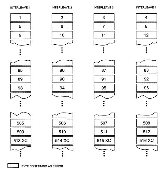
Figure 5-9 Twelve Correctable Random Burst Errors
