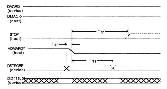
Figure 6-5 Host Pausing a Data In Burst
