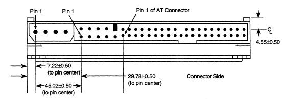
Figure 3-6 AT Connector and Jumper Location
