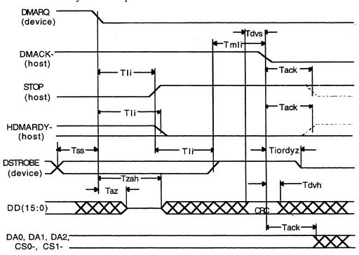
Figure 6-6 Device Terminating a Data In Burst
