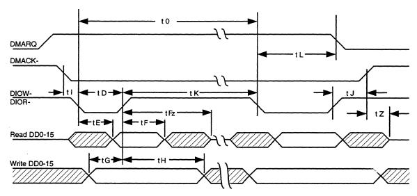
Figure 6-2 Multiword DMA Bus Interface Timing
