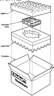
Figure 3-2 Drive Packing Assembly
