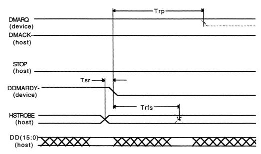
Figure 6-10 Device Pausing a Data Out Burst
