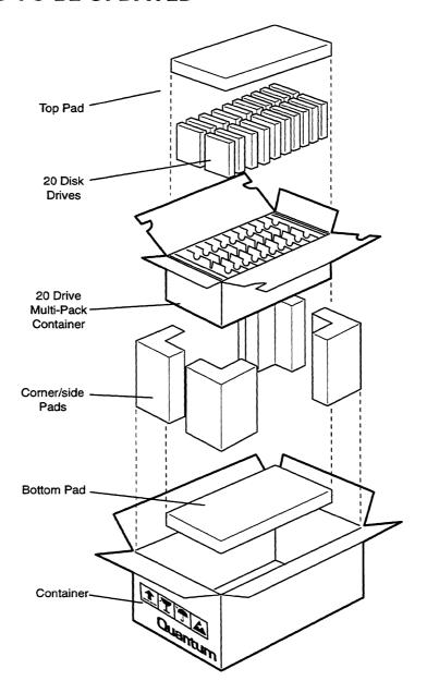
Figure 3-3 Drive Packing Assembly of a 20-Pack Container
