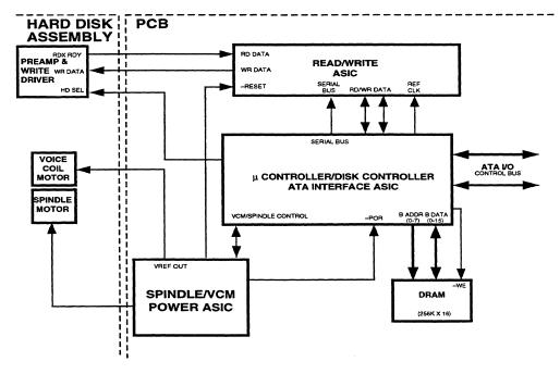
Figure 5-2 Quantum Fireball CR 4.3/6.4/8.4/12.7AT Hard Disk Drive Block Diagram
