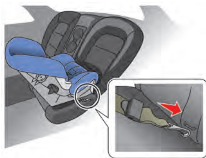
Rear-facing web-mounted — step 2
