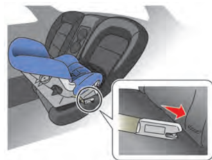
Rear-facing rigid-mounted — step 2
