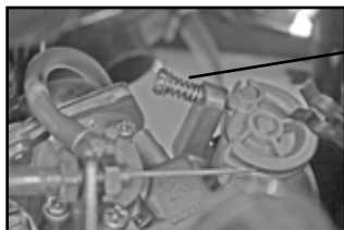
Engine Idle adjustment Screw
