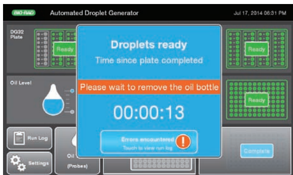
Fig. 20. Droplet generation is complete. Please wait to remove the oil bottle until the orange message disappears from the screen.
