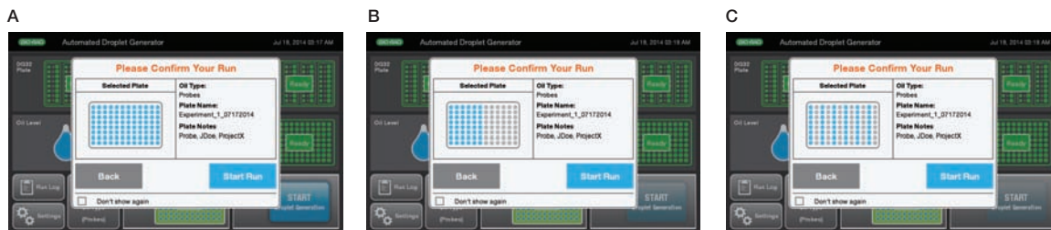
Fig. 15. Run confirmation screen. A, full plate of samples selected; B, half plate of samples selected; C, alternating columns of samples selected.
