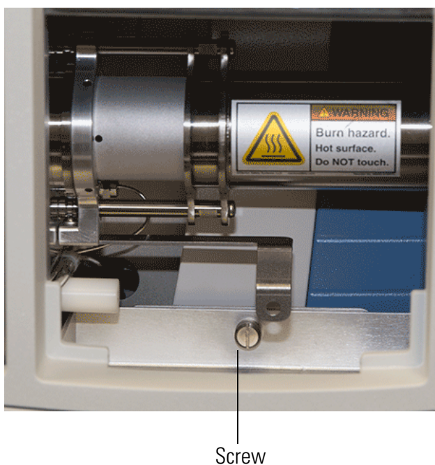
Figure 8-39. Locating the Back Screw
