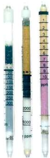
Figure 24: Example of chemical indicator tubes
