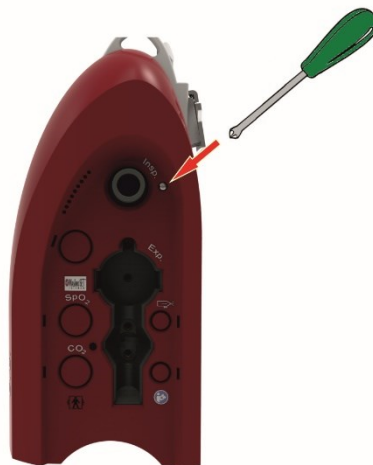
Fig. 118: Removing the screw on the side panel
