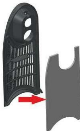
Fig. 116: Replacing the coarse filter
