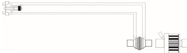
Fig. 70: Flow sensor connection with distal expiration valve
