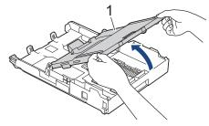
4. Load up to 10 envelopes in the paper tray with the printing surface **face down**. Loading more than 10 envelopes may cause paper jams.
