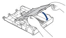
6. Load up to 20 sheets of photo paper with the printing surface **face down**. Loading more than 20 sheets of photo paper may cause paper jams.
