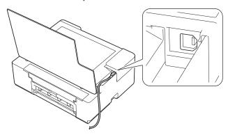
Carefully guide the cable through the cable channel and out the back of the machine.
