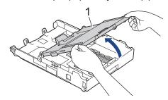
4. Gently press and slide the paper width guides (1) and then the paper length guide (2) to fit the paper size.
