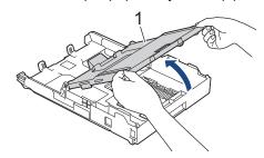
4. Gently press and slide the paper width guides (1) to fit the paper size, and then lift the stopper (2).
