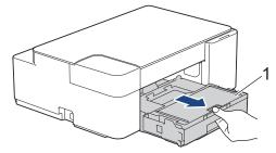
4. Clean the machine's printer platen (1) and the area around it, wiping off scattered ink with a dry, soft lint-free cloth.
