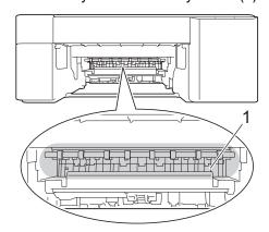
5. Push down on the Jam Clear Cover (1) on the back of the machine, and then open it (2).
