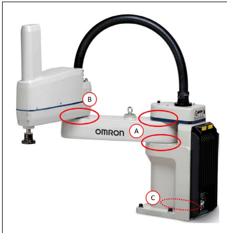
Figure 7-5. eCobra Oil Leak Inspection Areas
