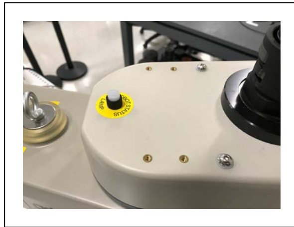
Figure 5-2. External Equipment Mounting location, J1
