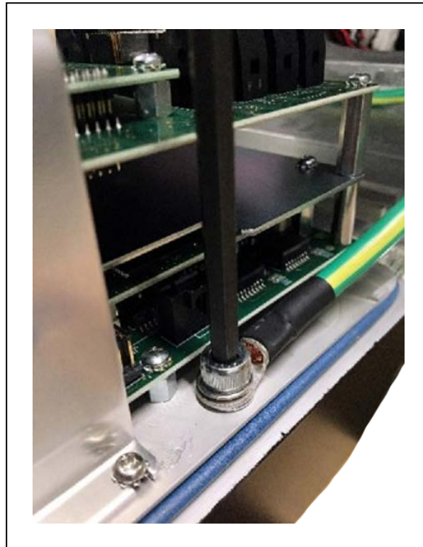
Figure 7-12. Removing Ground Screw Wire on iCS-ECAT Amplifier Chassis with 5 mm Hex Wrench
