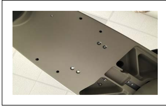
Figure 5-4. External Tooling Location, Outer Link (bottom)
