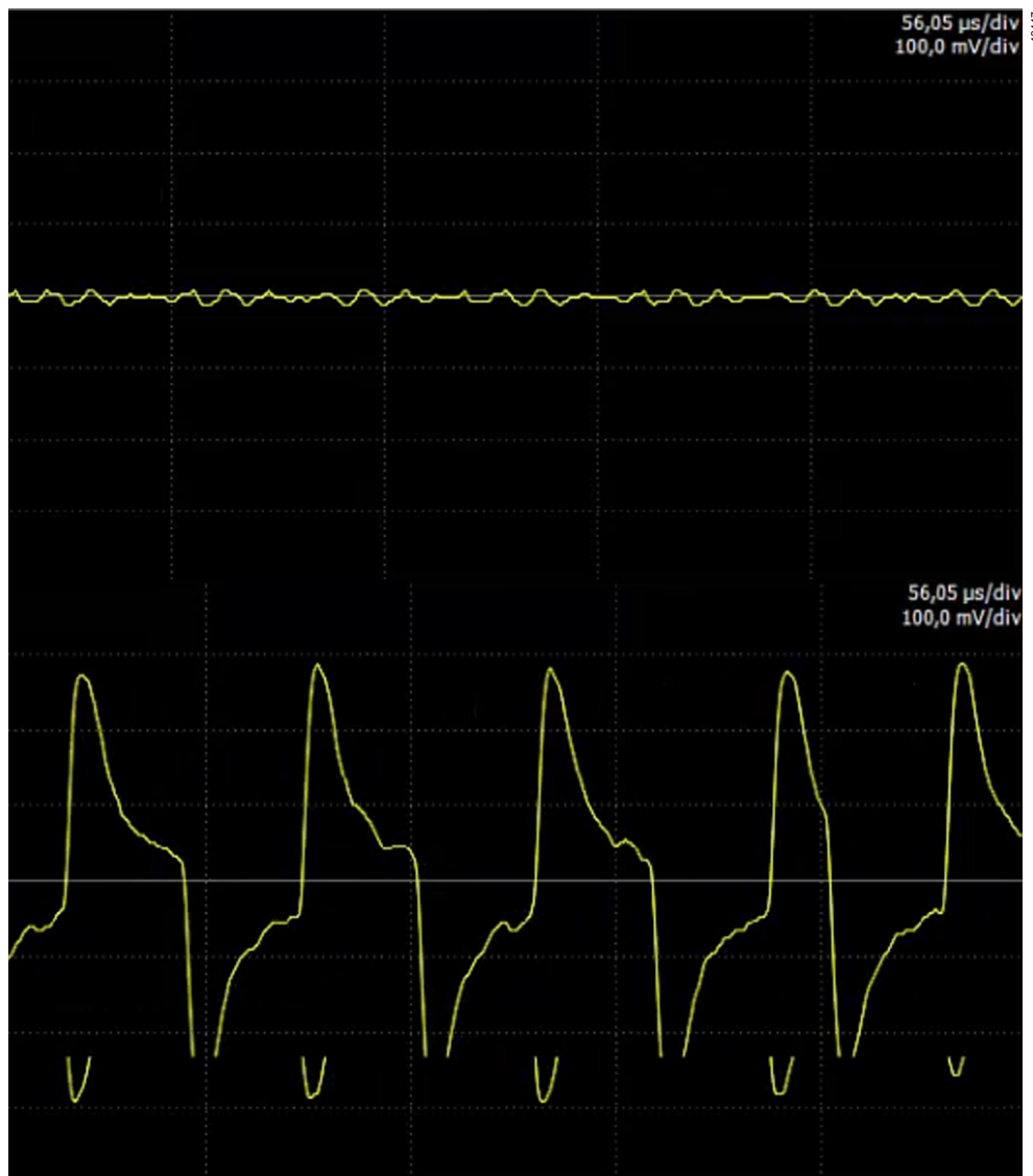
Fig. 6 Oscilloscope image of a bus segment with the connections the wrong way round
