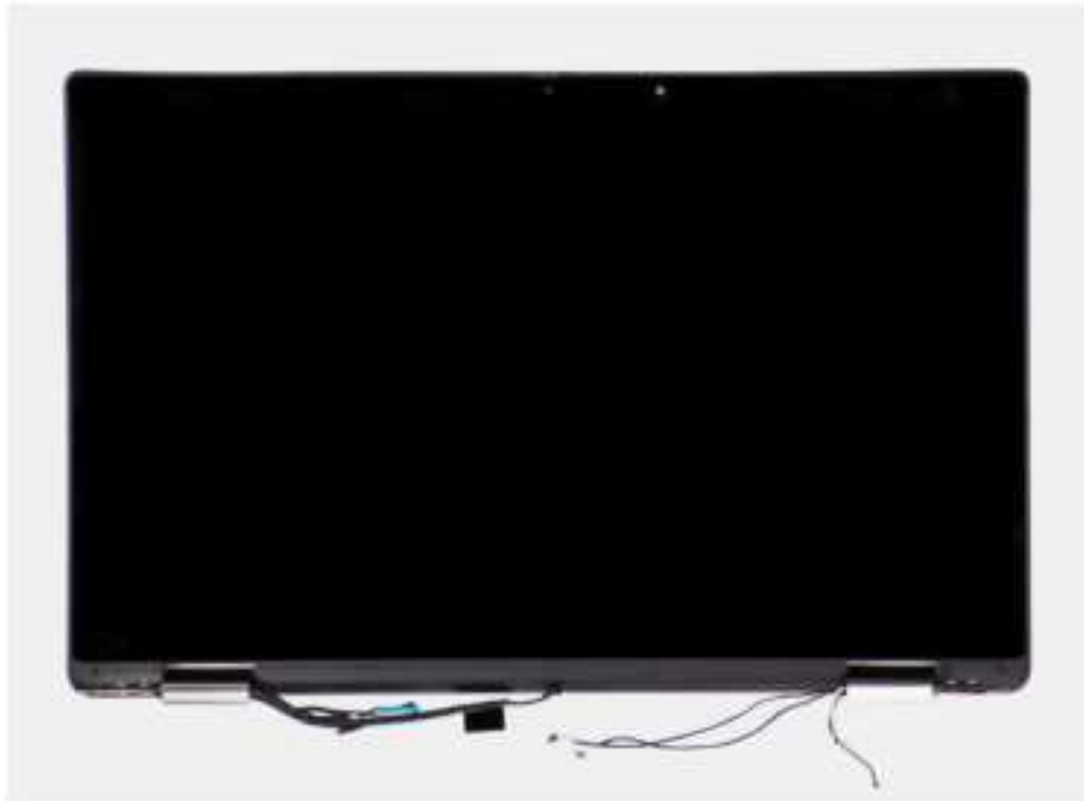
Figure 1. Display assembly with antennae cables
