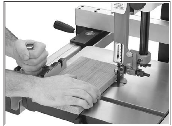
Figure 43. Making a 90° crosscut.
