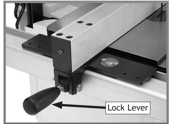
Figure 12. Fence secured in place.
