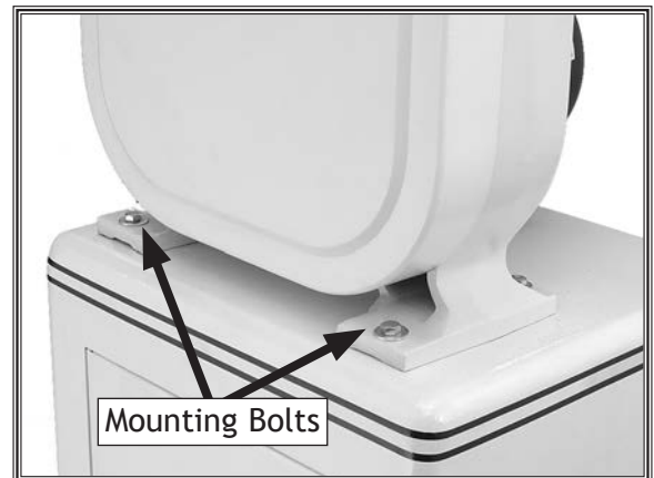
Figure 7. Bandsaw body mounted on the cabinet stand.
