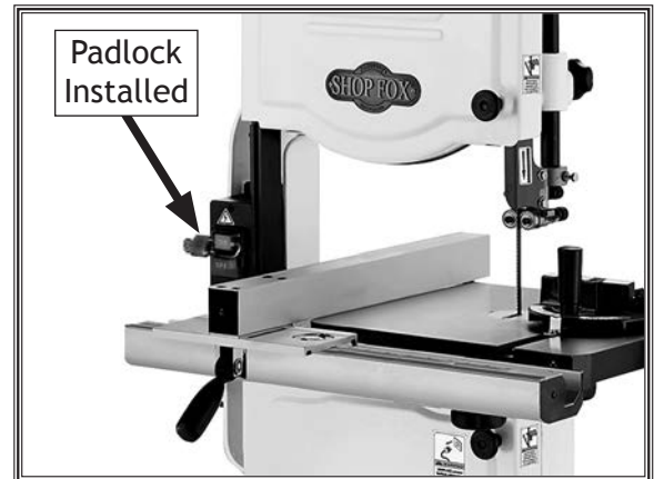
Figure 34. Padlock installed in the switch.
