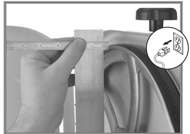
Figure 63. Measuring the distance the wheel is out of adjustment.
