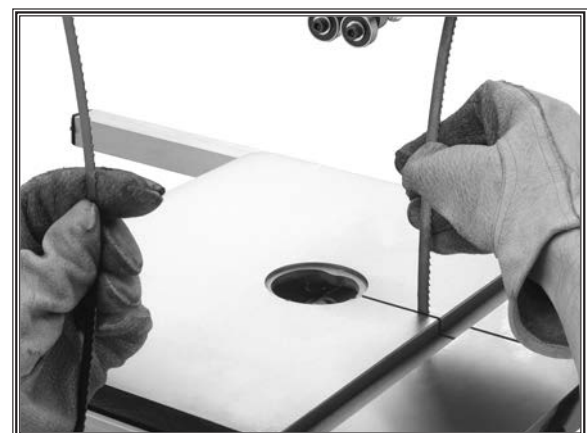
Figure 51. Changing the blade.
