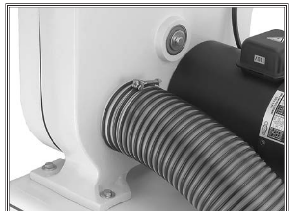
Figure 13. Dust collection hose connected to the dust port.
