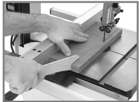
Figure 42. Example of ripping.
