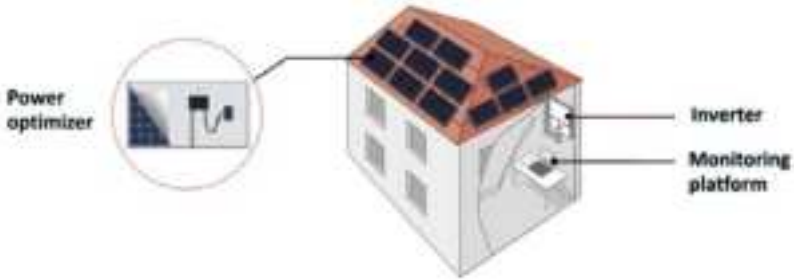
Figure 1: The SolarEdge power harvesting system components
