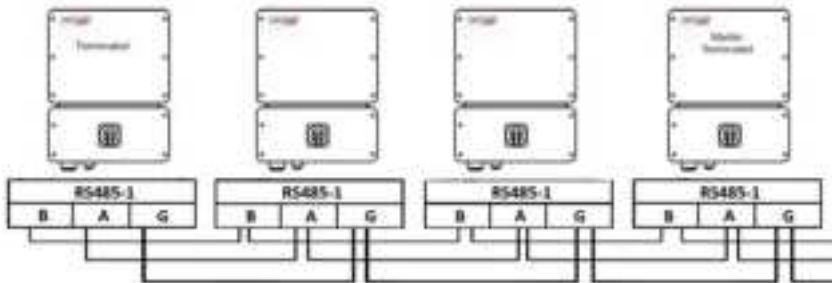
Figure 30: Connecting the inverters in a chain
