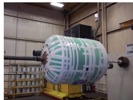
Insulated Vessel at Start of Winding
