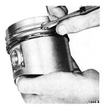
FIG. 64—Ring Side Clearance—Typical
