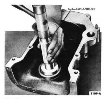
FIG. 41—Oil Seal Installation
