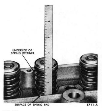
FIG. 25—Valve Spring Assembled Height
