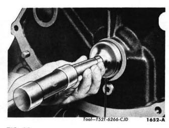
FIG. 39—Camshaft Rear Bearing Bore Plug Installation
