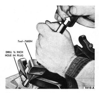
FIG. 29—Water Outlet Plug Removal
