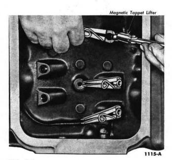
FIG. 47—Lifting and Securing Valve Tappets—
