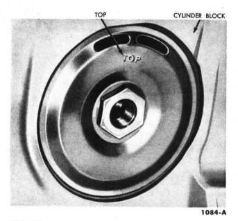
FIG. 71—Anti-Drain Back Diaphragm Position
