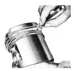
FIG. 47—Checking Ring Side Clearance
