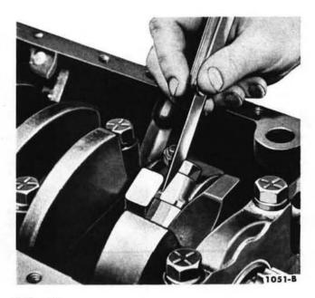
FIG. 44—Connecting Rod Side Clearance
