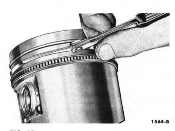
FIG. 42—Piston Ring Side Clearance
