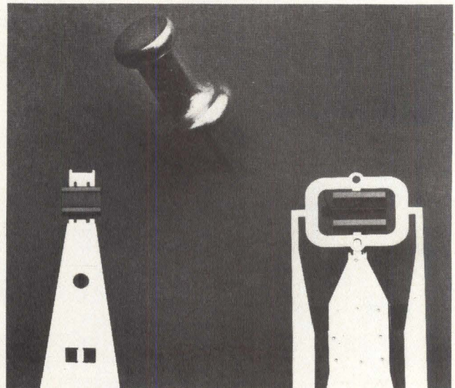
Figure 1: ST512s thin film head (left) provides mechanical and electrical characteristics superior to ferrite heads (right). Width of board track is 0.375".
