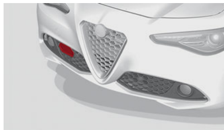
Front Bumper Radar Location
