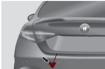
Manual Release Cord Shown With Trunk Closed
