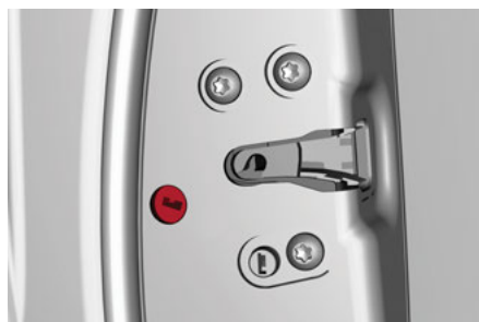
Door Lock Manual Release Lock Cylinder
