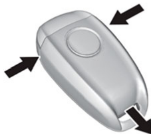
Emergency Key Release Buttons
