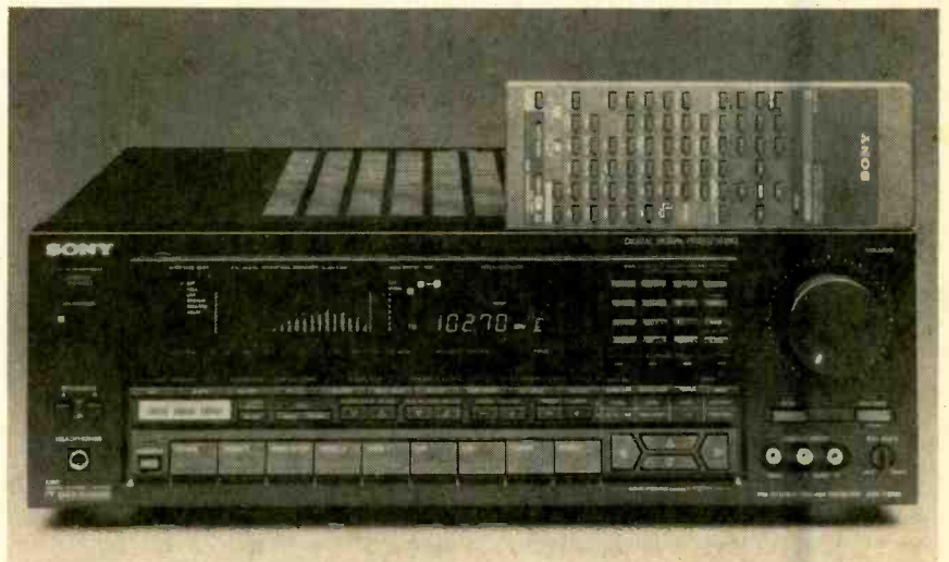
A receiver houses an amplifier, a preamp, and a tuner, all in one. Many modern receivers like this one, commonly called an A/V receiver, include surround-sound processors for video equipment.
