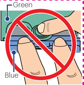
7 Slide the Black Ink cartridge all the way into the left slot using the green rail.
