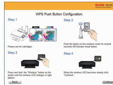
3 Press and hold
