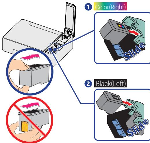
6 Slide the black ink cartridge all the way into the left slot using the green rail.
