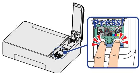
5 Slide the color ink cartridge all the way into the right slot using the green rail.
