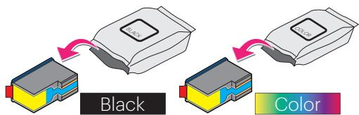
2 Remove the plastic tape on the black and color ink cartridges using the red pull tab.
