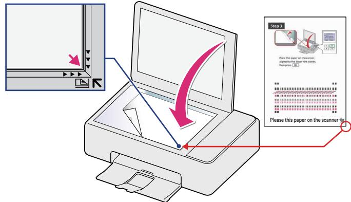
6 The unit will start scanning the alignment pattern to set an appropriate alignment on this unit.
