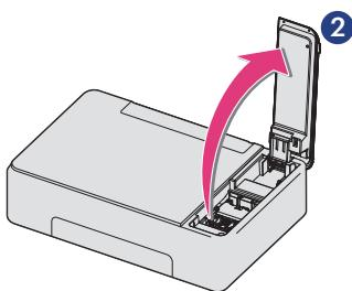
4 Press front side blue Cartridge tab with 2 fingers to open the cartridge slot.
