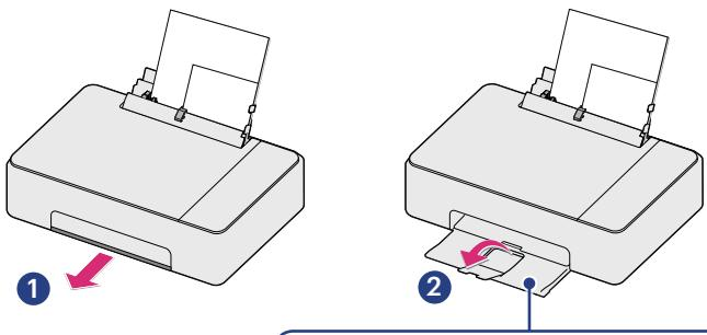
Pull out the Paper exit tray all the way before opening the Exit tray extender.
