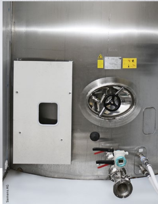
... and the pressure transmitter Sitrans P D S III in endurance tests
