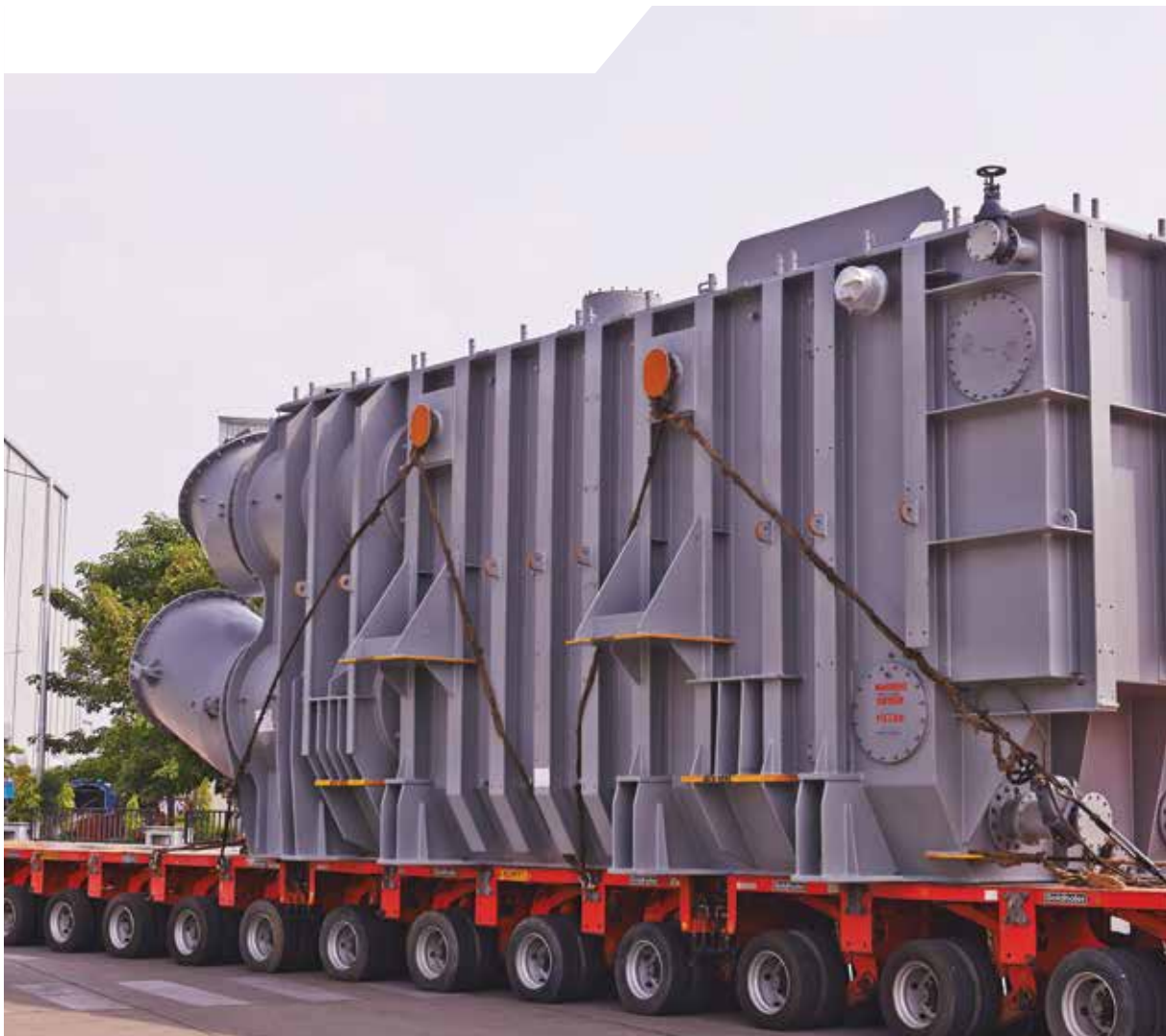
800kV UHVDC transformer successfully despatched for PowerGrid Champa Kurukshetra project from Vadodara
