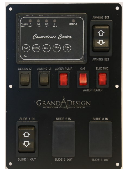
Typical Command Center, located inside the RV.
