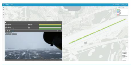
RoadAI makes it easy to collect, view, and leverage runway condition data on a map.
