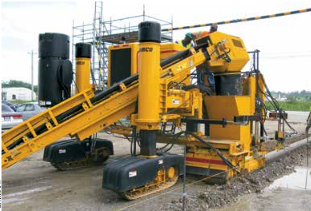
The GT-3600 uses the trim/pour feature on a unique curb profile.
