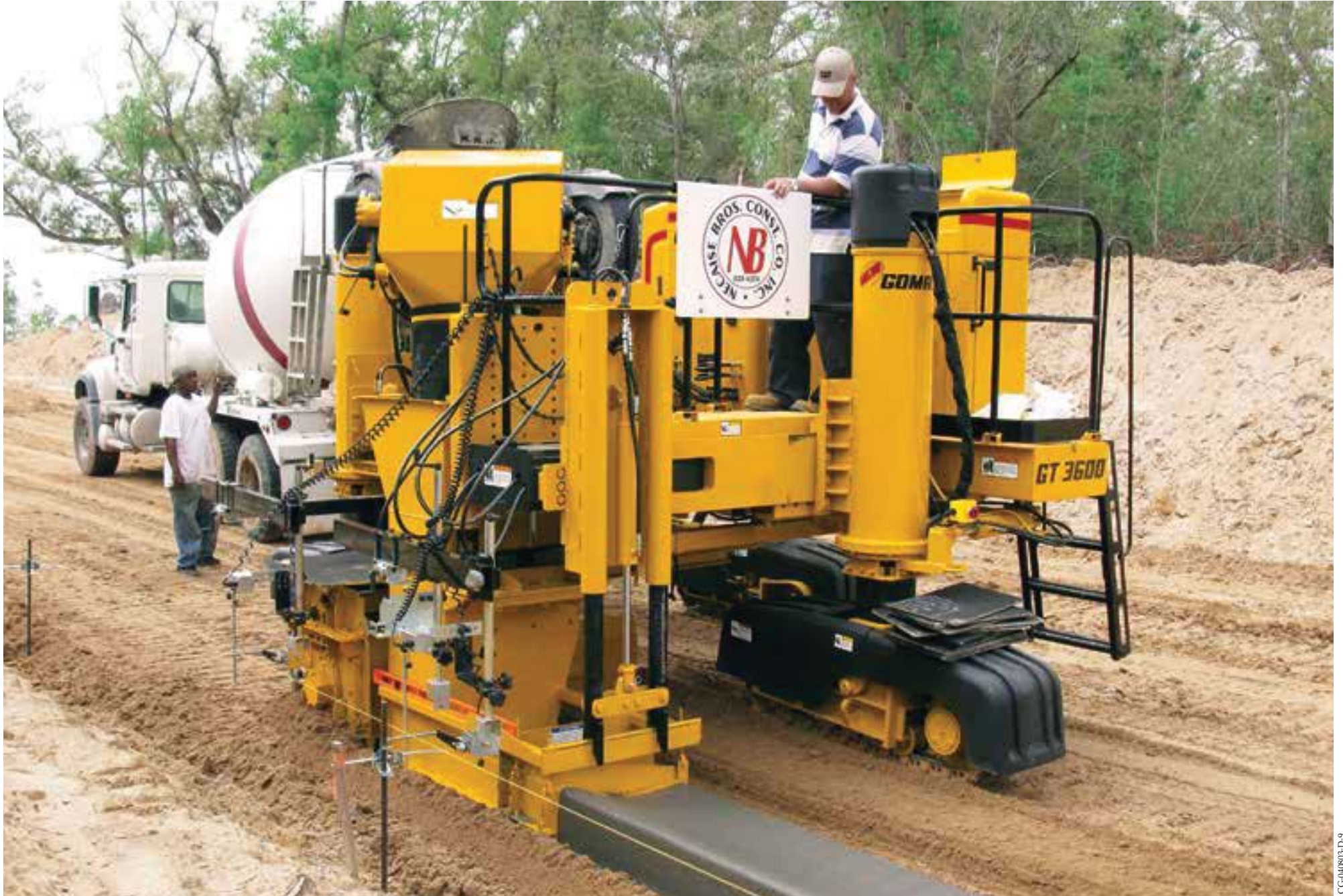
The GT-3600 has an operational speed up to 42 feet per minute (12.8 mpm) for high production curb and gutter slipforming applications.
