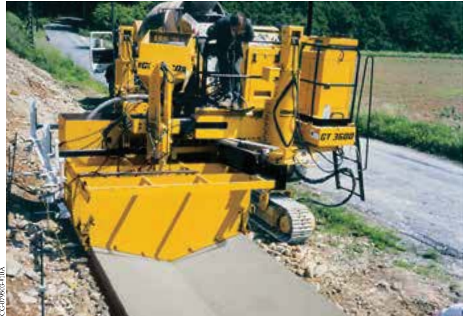
The versatile GOMACO GT-3600 slipforms a drainage channel in France. The side-mounted design allows minimum-clearance on the left side of the mold.
