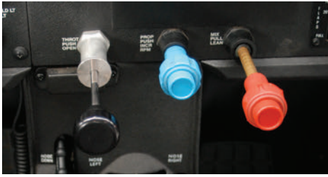
Figure 1-13 Push/pull knobs for throttle, propeller and mixture controls (Cessna aircraft).
