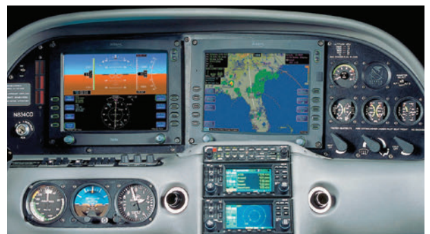
Figure 1-33 Cirrus instrument panel showing the primary flight display (PFD) and multi function display (MFD).
