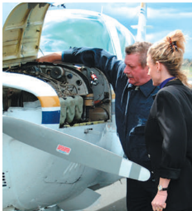
Figure 1-17 The oil quantity should be checked during the preflight inspection prior to every flight.
