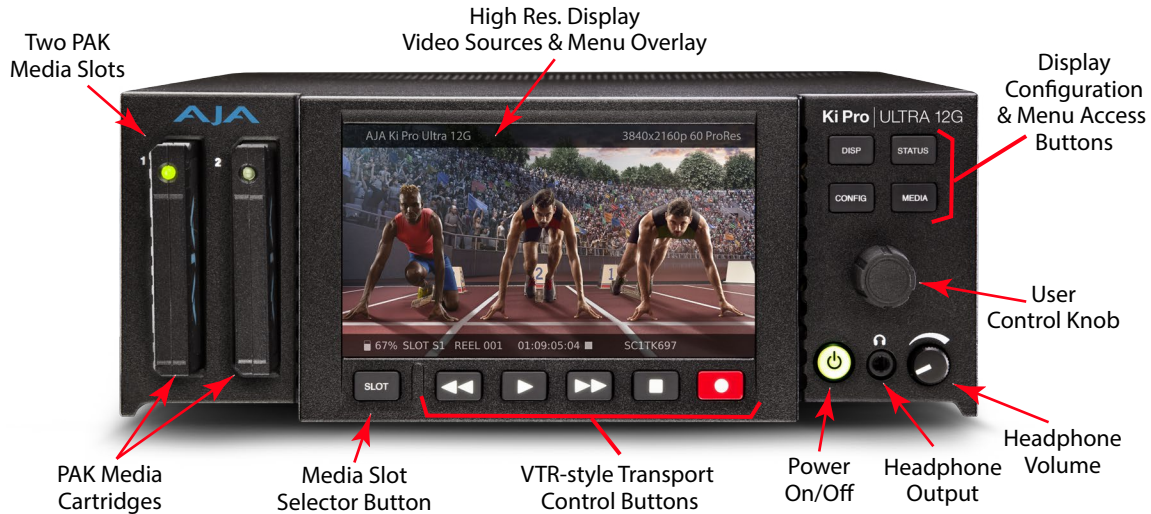
Figure 1. Ki Pro Ultra 12G Operator Side Controls
