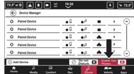
Uconnect 5/5 NAV With 10.1-inch Display Or 12-inch Display Two Active Phones Button
