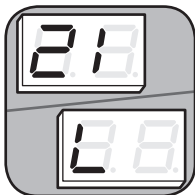
Active Protection – Code 21L – Open low-pressure control
