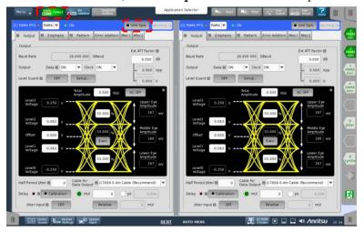
Observe the outputs (total 8 channels) of MU196020As installed in Master and Slave with an oscilloscope, and you can now confirm that the bit phase difference of each channel is within  $\pm 1024$  UI.
