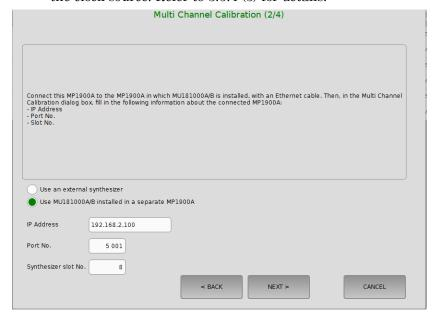
Figure 3.5.2-5 Multi Channel Calibration Dialog Box 2/4
