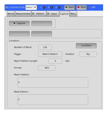
Figure 4.3.4.5-1 MU195040A Capture Tab
