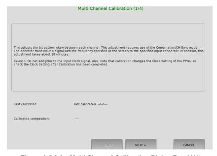
Figure 3.5.2-3 Multi Channel Calibration Dialog Box (1/4)
