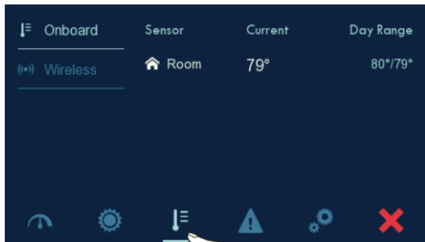
This page displays sensor information. Select 'Onboard' to view room temperature sensors that are built-into the thermostat. Select 'Wireless' to view all wireless sensors that this thermostat has access to.
