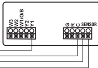
Free Cooling utilizes the Y1 terminal for the operation of 1st stage cooling. If mechanical (compressor) cooling is also present, the mechanical cooling is connected to the Y2 terminal in this instance.
