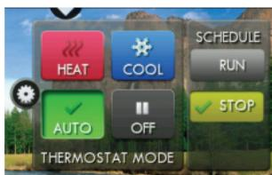
**AUTO-CHANGEOVER MODE** - Pressing the WARMER or COOLER buttons in Auto mode will adjust both the heat and cool setpoints simultaneously. To adjust heat and cool setpoints individually, choose HEAT mode to adjust the heat setpoint and COOL mode to adjust the cool setpoint, then return to AUTO mode.
