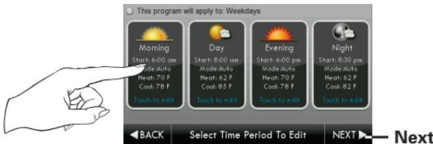
Adjust Mode, Start Time, and Heat and Cool Setpoints to desired settings. The Time Period may also be Enabled or Disabled. Un-check the Enabled box for Time Periods you don't want to use. Press **DONE** when finished.
