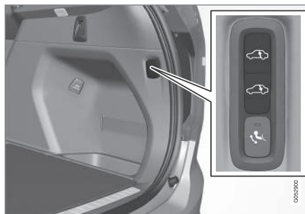
Controls for raising/lowering the car's rear section.
