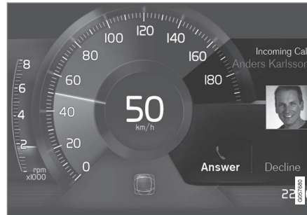
Example of message in the 8-inch driver display. The figure is schematic - parts may vary depending on car model.
