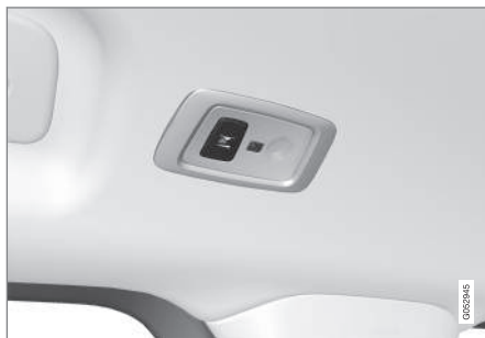
In cars with panoramic roof* there are two lamp units, one on each side of the roof. 10
