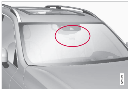
Radar unit location
