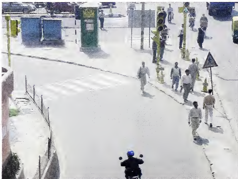
Fig. 5.15 Channelisation Providing Refuge to Pedestrians
