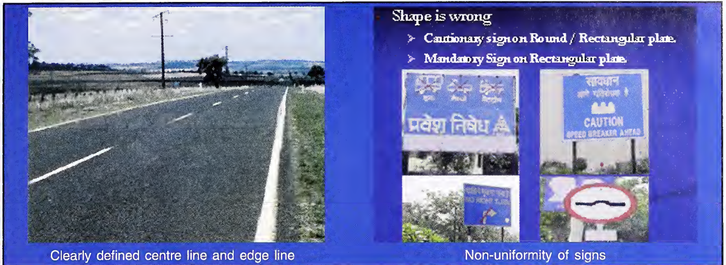
Fig. 5.27 Traffic Control Devices for Better Road Safety
