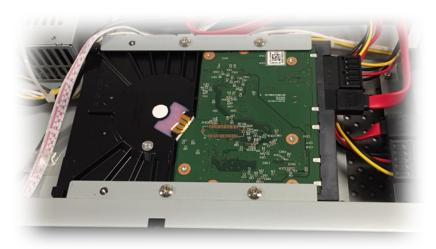
Remove the four screws that hold the hard drive in place and carefully slide the hard drive out.
