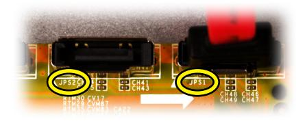
Be sure to connect them in the correct order. Looking at the recorder from the front of the unit, the SATA ports are numbered and 2. Looking closely at the board, you can actually read the numbers beside each port after the letters *JPS*.
