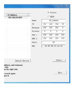
Check the camera data at the top of the right column. It may be that the camera is set to a static IP, and this static IP address is incompatible with your system's subnet address (see the example at left).
