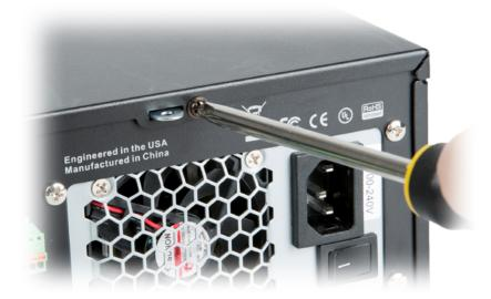
Using the thumb notch on the top of the unit, gently slide the cover about an inch to the rear of the unit, then lift it up. Once it is off, set the lid aside in a safe place where it won't get scratched.
