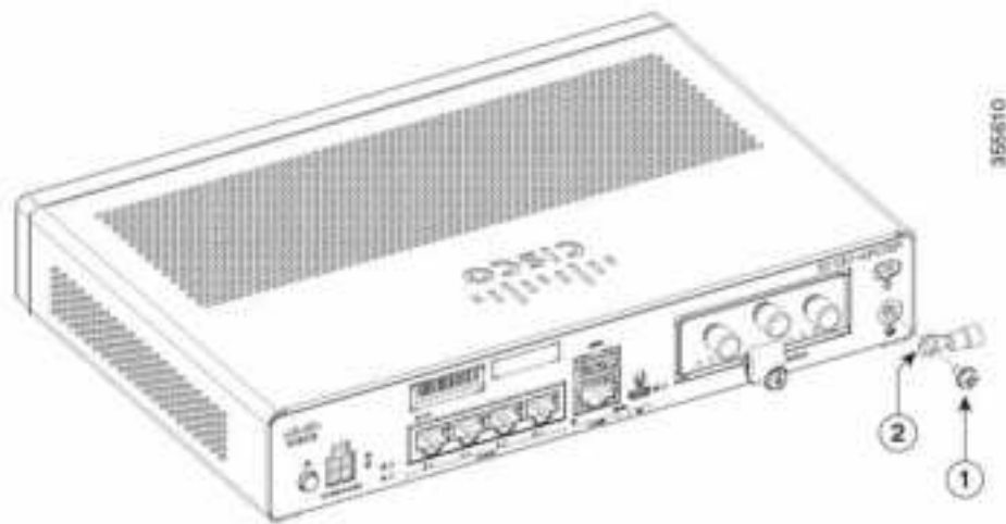
Figure 53: Chassis Ground Connection-Cisco 1101-4PLTEP
