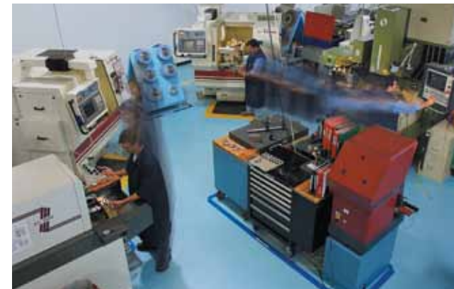
Cellular manufacturing streamlines operations and achieves one-piece flow by allowing team members to complete multiple operations.
