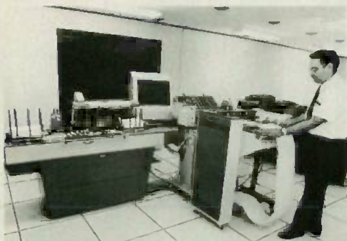
E-COM EQUIPMENT UNDER TEST at the RCA Government Communications System, Camden, NJ. (RCA supplied the equipment for the new system, on a $31-million contract.) The system accepts inputs from a customer's computer-generated magnetic tape or from a computer via private telecommunications carriers and transmits it to the electronic center designated by the customer, where it is printed, trimmed, folded, placed in envelopes, and delivered by first-class mail.
