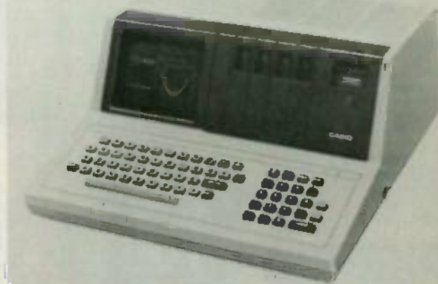
THE CASIO FX-9000P personal computer. The basic unit comes with a 4K RAM, a 9.5-inch built-in CRT, very extensive high-resolution graphics, and powerful mathematical functions for scientific, engineering and statistical operations.
