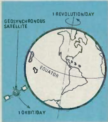
FIG. 1—THE ORBITAL VELOCITY of a geosynchronous satellite matches the rotational speed of Earth exactly, making it appear to be stationary in the sky.
