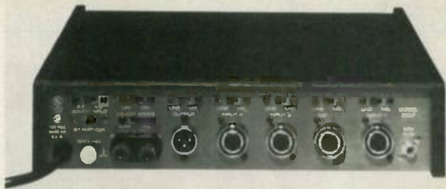
FIG. 1—A MIXER, such as the Shure M267, allows you to use several microphones or other audio sources.
