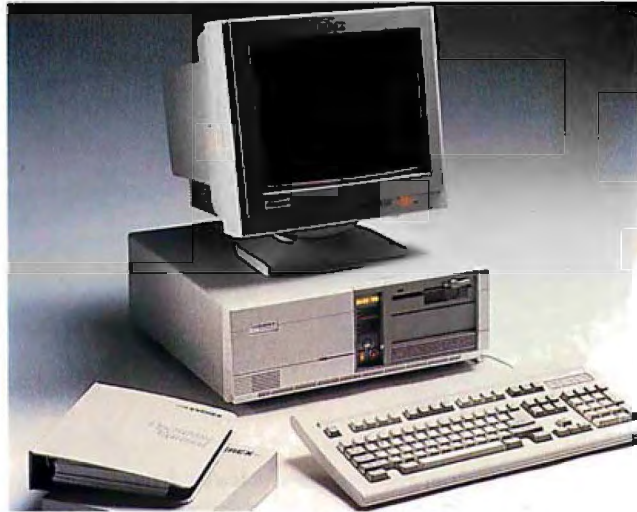
Everex's Step 386is is built around Intel's 386SX.
