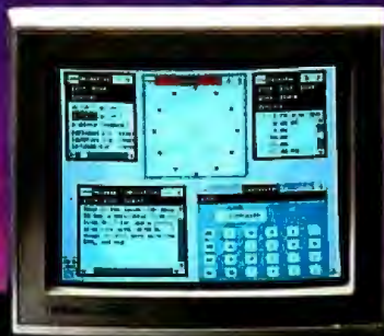
MultiVision 770+. A 14-inch multi-sync with CGA, EGA, VGA and up to 800 x 600 resolution.
