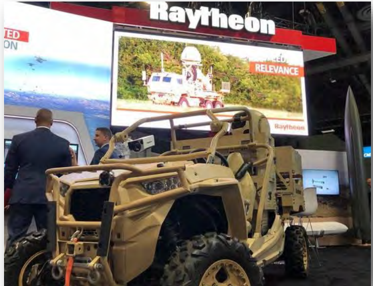
RAYTHEON'S HIGH-ENERGY LASER COUNTER-DRONE SYSTEM IS MOUNTED ON A POLARIS MRZR ALL-TERRAIN VEHICLE AT THE ASSOCIATION OF THE UNITED STATES ARMY'S ANNUAL MEETING IN WASHINGTON, D.C., IN OCTOBER 2019. PHOTO BY HOPE HODGE SECK.
