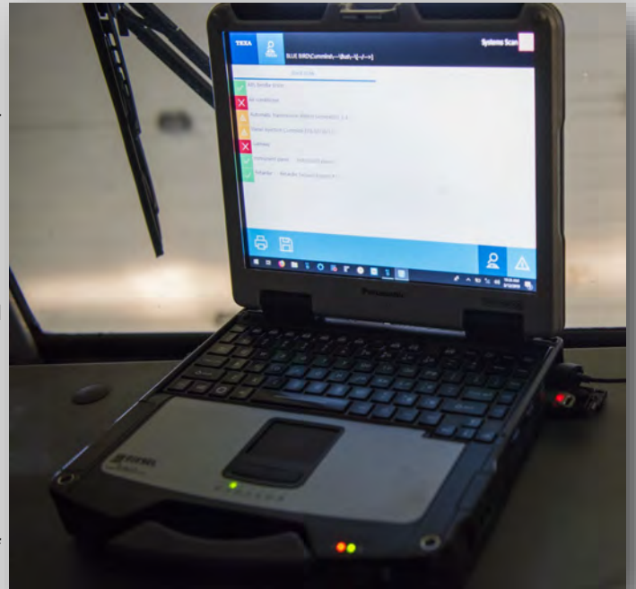
The new proprietary vehicle diagnostic tool at Mountain Home Air Force Base, Idaho, replaces the need for having multiple tools for different types of vehicles. This saves resources by eliminating the need to outsource maintenance. (U.S. Air Force photo by Airman 1st Class Andrew Kobialka)
