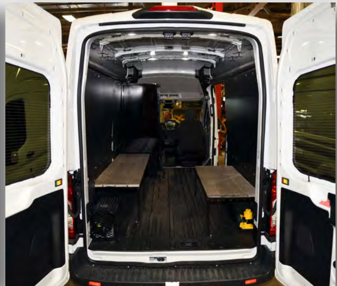
The bread trucks, now insulated for warmth, provide technicians with transportation at Ellsworth Air Force Base, S.D., Jan. 3, 2019. Two of the five trucks have insulation installed, now only requiring the tool cages and benches. (U.S. Air Force photo by Senior Airman Donald C. Knechtel)
