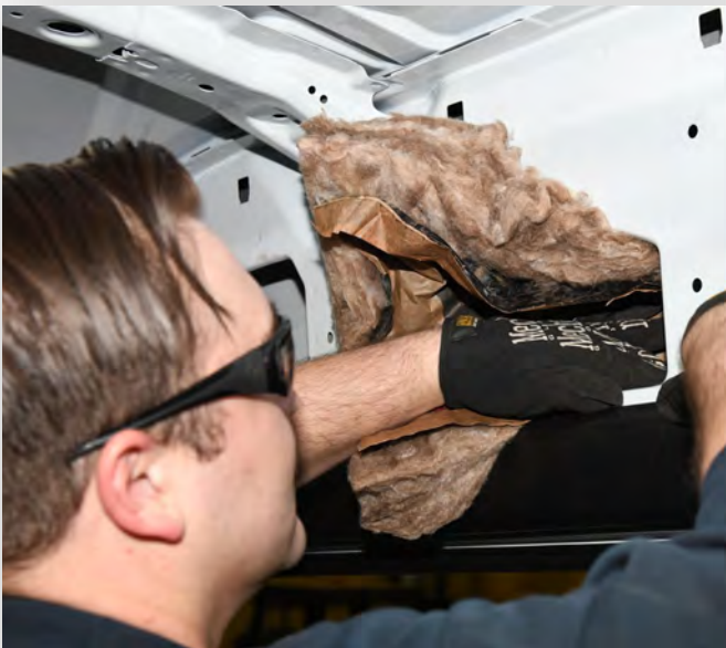
Senior Airman Kyle Nauman, a 28th Logistics Readiness Squadron vehicle maintenance equipment technician, installs insulation to the side of a bread truck at Ellsworth Air Force Base, S.D., Jan. 3, 2019. The new insulation will now help maintainers and technicians keep warm during the harsh winters while transporting to and from the fight line. (U.S. Air Force photo by Senior Airman Donald C. Knechtel)
