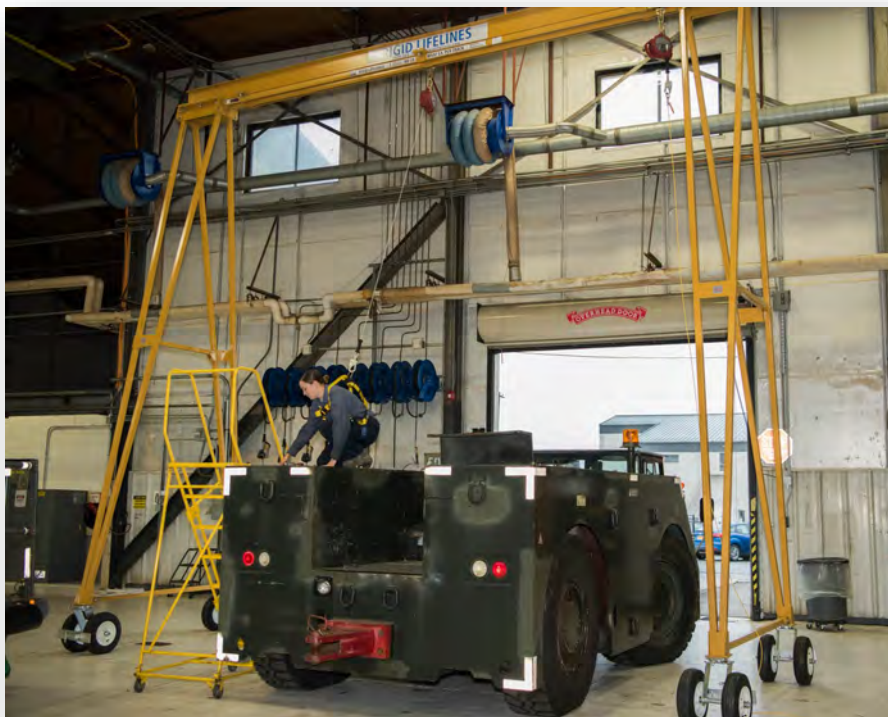
AIRMAN 1ST CLASS KILEY GRING, 436TH LOGISTICS READINESS SQUADRON MULTIPURPOSE VEHICLE MECHANIC, OPERATES ON TOP OF A B-1000 AIRCRAFT TOW TRACTOR NOV. 6, 2018, AT DOVER AIR FORCE BASE, DEL. GRING WORE A BODY HARNESS CONNECTED TO THE LRS'S NEW MOBILE "A-FRAME" FALL-PROTECTION SYSTEM, WHICH PREVENTED HER FROM FALLING ON THE JOB. (U.S. AIR FORCE PHOTO BY STAFF SGT. ZOE RUSSELL)
