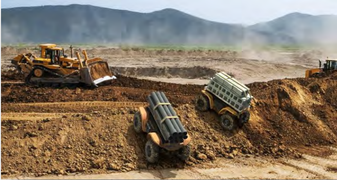
In construction applications, the Autonomous Work Vehicle could be used to transport heavy materials. Photo courtesy of Honda
