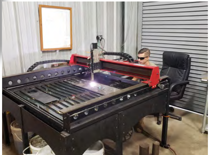
Army SGT Clark Millikan demonstrates the shop's plasma cutter
