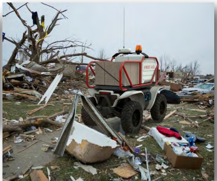
The autonomous vehicle prototype could be programmed to transport heavy materials during emergency situations, lowering the risk of injury for first responders. Photo courtesy of Honda
