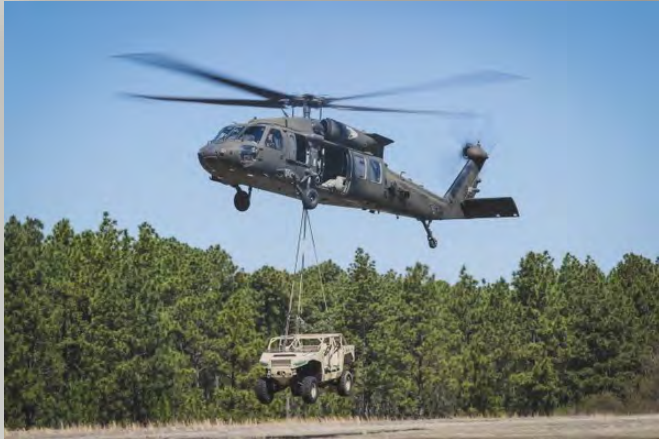
A UH-60 BLACK HAWK HELICOPTER ASSIGNED TO THE 2ND ASSAULT HELICOPTER BATTALION, 82ND COMBAT AVIATION BRIGADE, LIFTS A POLARIS DAGOR IN SUPPORT OF THE XVIII AIRBORNE CORPS' DEGLOPPER AIR ASSAULT SCHOOL ON FORT BRAGG, N.C., MAR. 23, 2017. (CAPT. ADAN CAZAREZ/ARMY)
