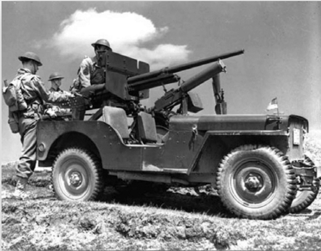
A TANK-KILLING JEEP IS EQUIPPED WITH A 37-MM GUN. (IMAGE SOURCE: WIKICOMMONS)
