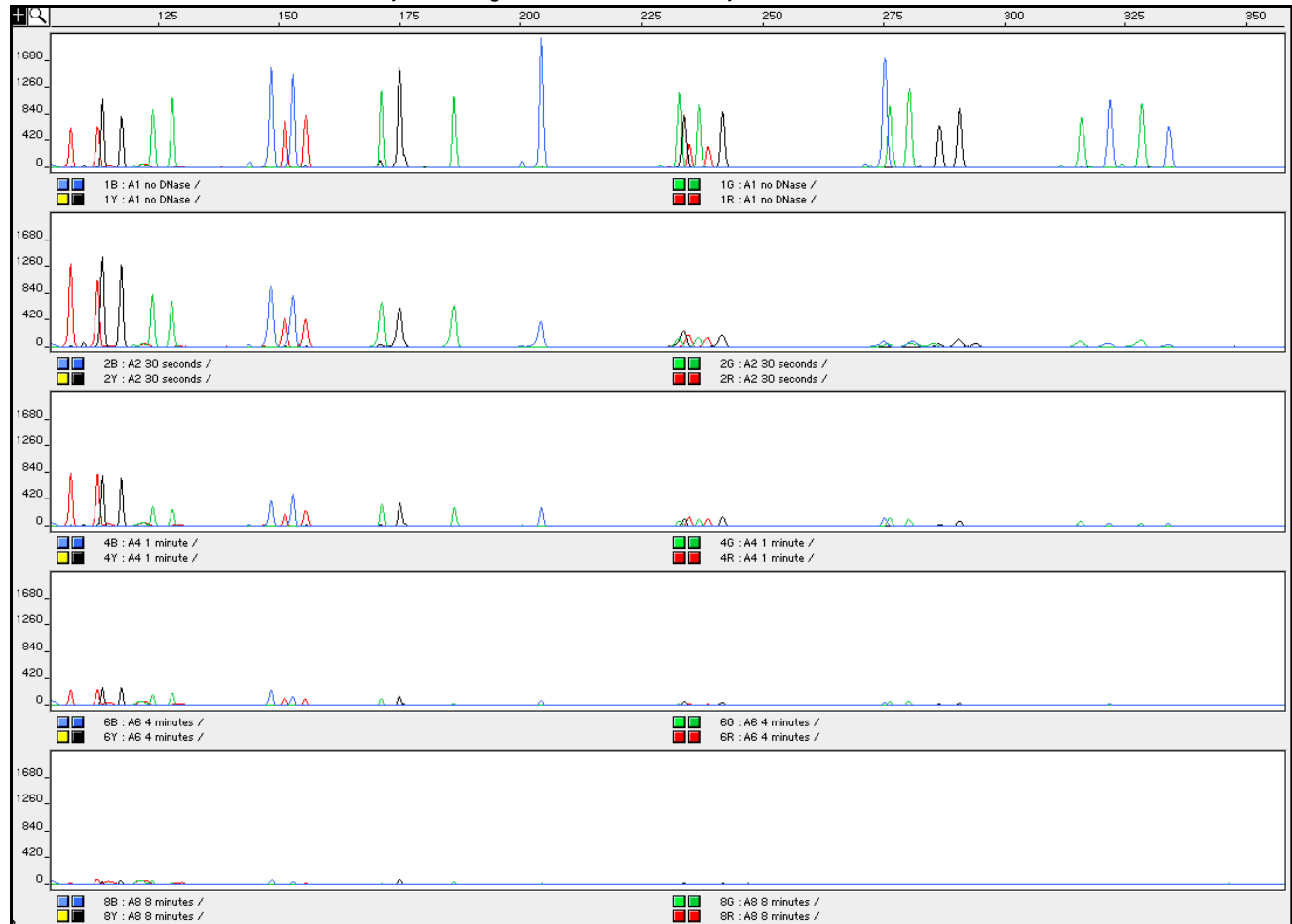
Figure 18 Multiplex amplifications of a DNA sample in the absence of DNase I and the sample incubated for 30 sec, 1 min, 4 min, and 8 min with DNase I, analyzed using the 310 Genetic Analyzer
