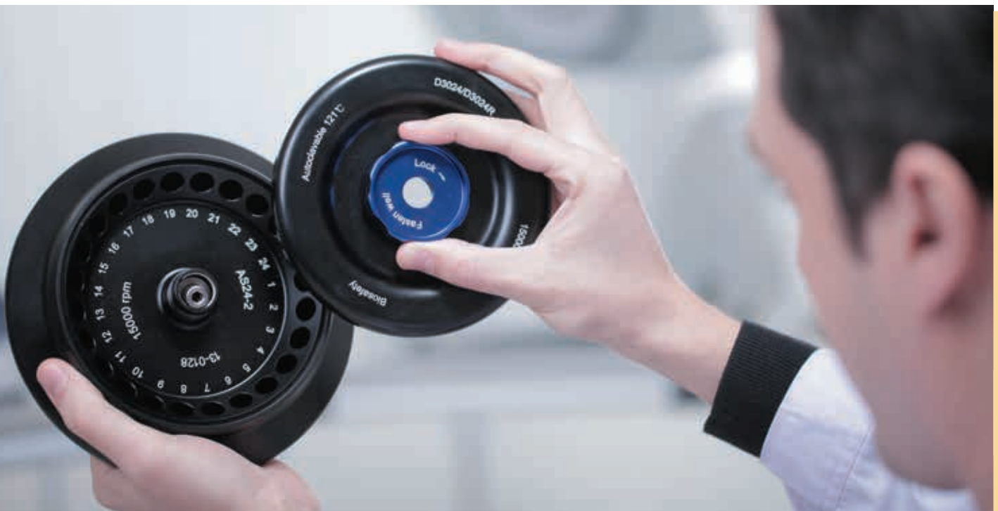
Seals within the aluminum alloy rotor
