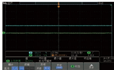
CV 50V high speed mode: CV stability, no vibration phenomenon
