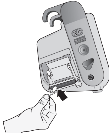
Figure 24-3. Cleaning the Print Head
