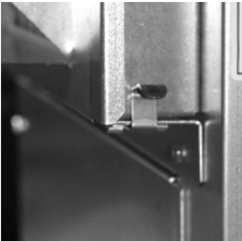
Figure 8 - Filter Rack Closed with Clip
