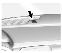
The security light, on the instrument panel near the windshield, indicates the status of the system:
