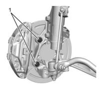
Apply liquid thread adhesive to the caliper bolts (GM Part No. 9985399 – Loctite 272 –
