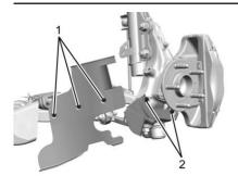
Install the small splash shields with two screws (2) per corner. Torque to 9 N•m (80 lb inch).
