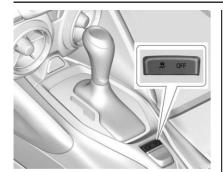
This optional handling mode can be selected by pressing the TCS/ StabiliTrak/ESC button on the console two times. The appropriate message displays in the Driver Information Center (DIC).
