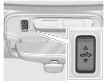
Press and hold the bottom of . The windows will automatically lower.  After the convertible top is completely open, a Driver Information Center (DIC) message displays. Release the switch.
