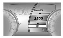
Press SEL to confirm the desired RPM.
