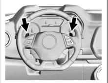
Tap Shift allows you to manually control the automatic transmission. To use Tap Shift, the shift lever must be in DSC mode. Vehicles with this feature have indicators on the steering wheel. The paddles are on the back of the steering wheel. Tap the left paddle (-) to downshift, and the right paddle (+) to upshift. The
