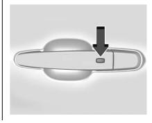
The RKE transmitter must be within 1 m (3 ft) of the trunk or door being opened. Press the button on the door handle to open. See "Keyless Access Operation" in *Remote Keyless Entry (RKE) System Operation* ⇒ 8.
