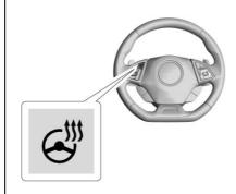
: If equipped, press to turn the heated steering wheel on or off. A light next to the button displays when the feature is turned on. The steering wheel takes about three minutes to be fully heated.
