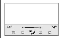
The climate control status display appears briefly when the center stack climate controls are adjusted.
