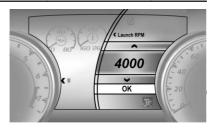
8. Adjust the desired RPM using  $\triangle$  or  $\nabla$ :
