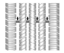
Treadwear indicators are one way to tell when it is time for new tires. Treadwear indicators appear when the tires have only 1.6 mm (1/16 in) or less of tread remaining. See *Tire Inspection* ⇔ 274 and *Tire Rotation* ⇔ 274.
