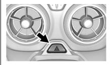
: Press to make the front and rear turn signal lamps flash on and off. This warns others that you are having trouble. Press again to turn the flashers off.
