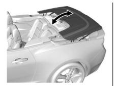
On each side of the tonneau cover, lift and pivot rearward into the fully open position. Hold the front and rear of the tonneau cover at the same time.
