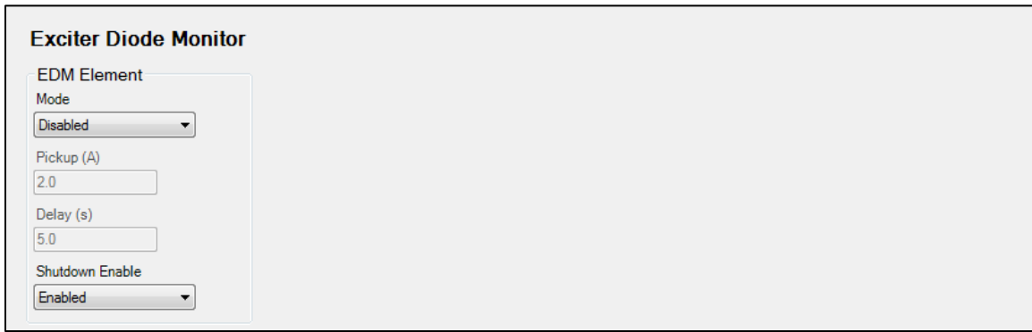
Figure 8-8. Exciter Diode Monitor Screen
