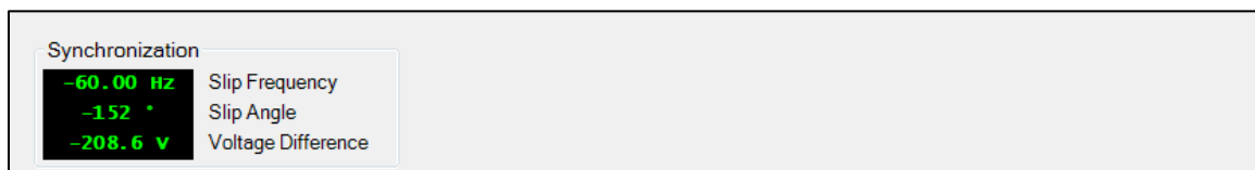
Figure 11-8. Synchronization Primary-Values Metering
