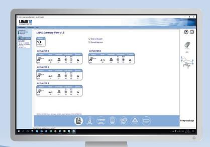
**Service Data Tool (SDT)** makes it possible to read out service data from the OpenBus<sup>™</sup> control box by informing about the use of the actuator system. SDT acts as preventive maintenance by disclosing wear and tear long before the system fails. This ensures minimal downtime as maintenance can be scheduled in due time. Efficient maintenance also helps prevent misuse, thus prolonging the equipment life.
