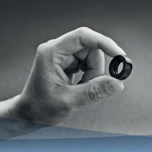
**Safety nut:** A safety nut acts as a precaution against potential failure of the main nut. If the main nut breaks, the safety nut will immediately carry the full load and thereby prevent potentially harmful falling.
